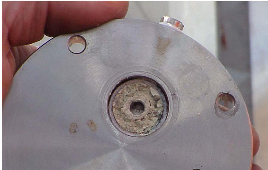
**Figure 7 – Sulfur on Particulate Filter After Process Upset**
